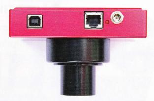
Left: The Infinity's ¾-inch format Sony ICX825 EXview HAD CCD II detector boasts high quantum efficiency, meaning you'll record faint objects with fairly short exposures. Right: Three ports on the bottom of the Infinity are a B-type USB 2.0, an RJ-12 port that allows the camera to be used as an autoguider, and a DC power input. The red LED is activated only when the camera is connected to your telescope mount.
