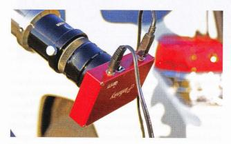
The camera's power cable port was very loose, often allowing the cable to fall out when slewing the telescope. A simple fix was to mount the Infinity upside down in the focuser.
